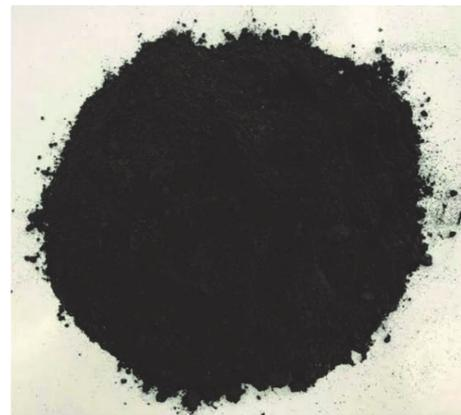
Fig. 2: Pyrolysis char from waste tyres
