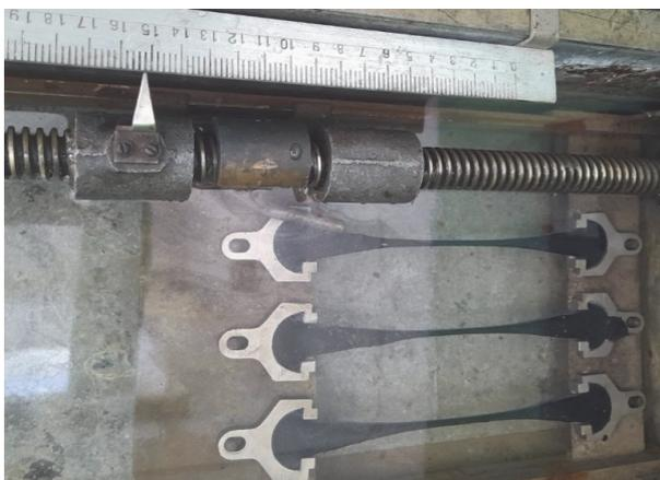
Figure 3. Determination of the bitumen extensibility (ductility)
