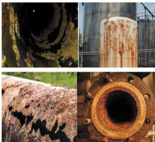
Figure 2. Different forms of Corrosion [45]
