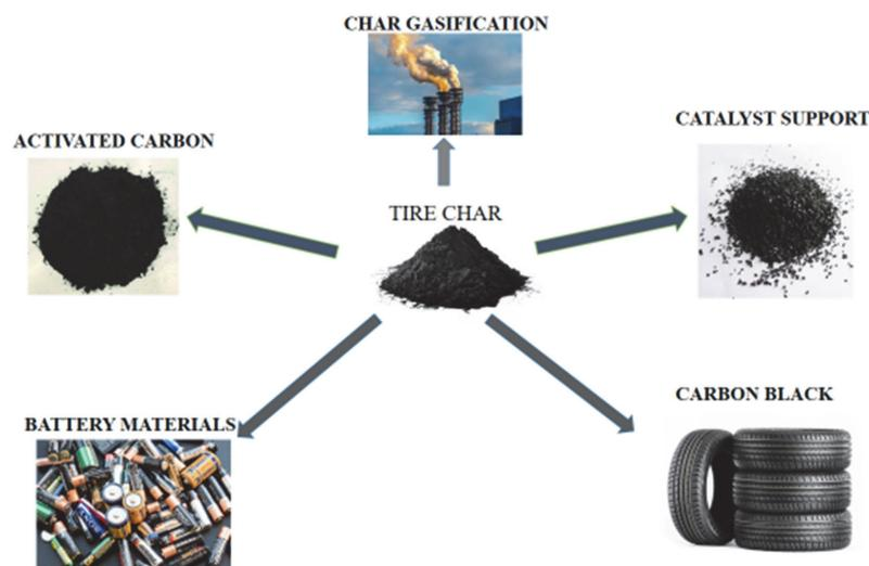
Fig. 4: The main high added value application of tyre char
