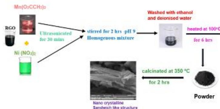
Figure 1. Schematic representation of synthesis procedure of RGO/NiO/MnO<sub>2</sub> nanocomposite
