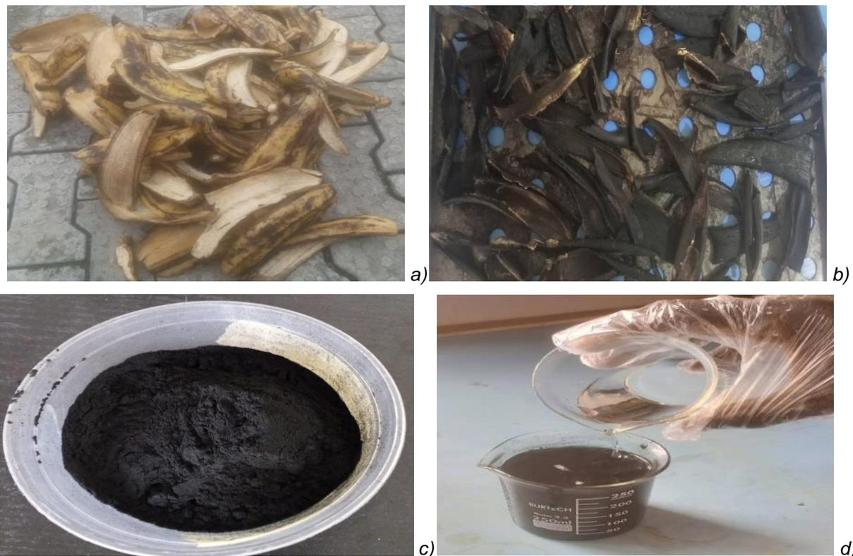
Figure 2. The Activated carbon preparation process (a) ripe plantain peel, (b) carbonized plantain peel, (c) activation of carbonised plantain peel carbon (d) activated plantain peel carbon.
