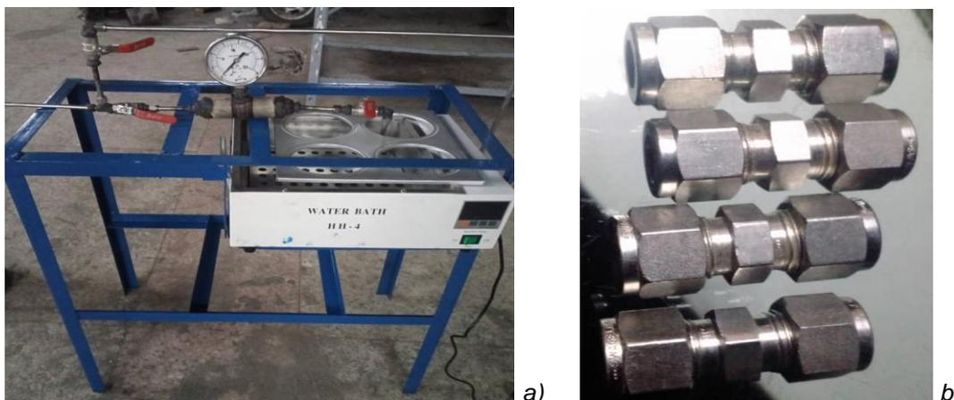
Figure 3. CO<sub>2</sub> adsorption equipment (a) Experimental setup for evaluation of CO<sub>2</sub> adsorption capacity (b) Reactors for storing adsorbents
