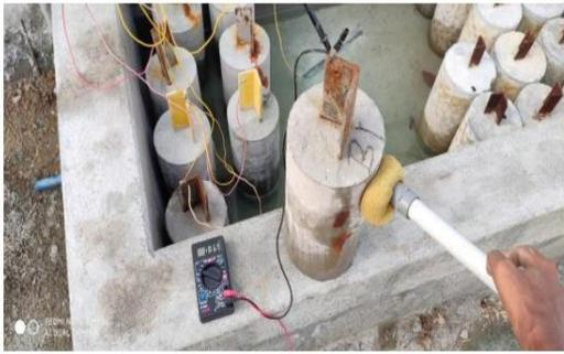
Figure 1. (b) HCP test on corroded specimen
