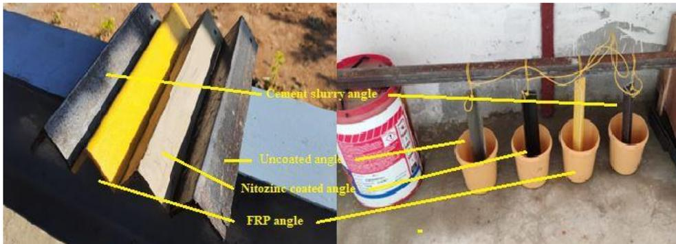
Figure 2. Applied Voltage Test – Setup
