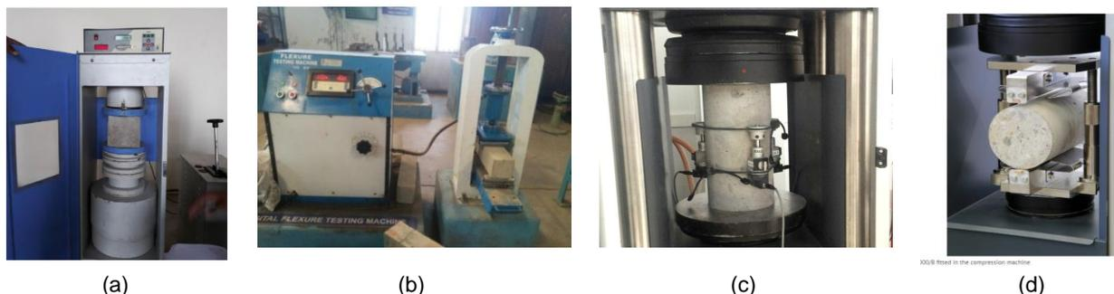
Figure 2. (a) Compressive strength test (b) Flexural strength test (c) Modulus of elasticity test (d) Split tensile strength test
