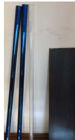
Figure 6 - Multilayered selective coating on PC tubes (on the left: two coated tubes vs. uncoated tube) and coated PC plate (on the right)
