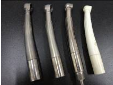
Figure 3 - Polyetherimide dental tools. Ti-coated (the first three samples from the left side) vs. uncoated tool (one sample on the right side)
