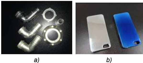
Figure 4 - PET samples coated with: a) Ti- PVD deposited coatings for different purposes, b) TiO_2 deposited coatings for decorative purpose
