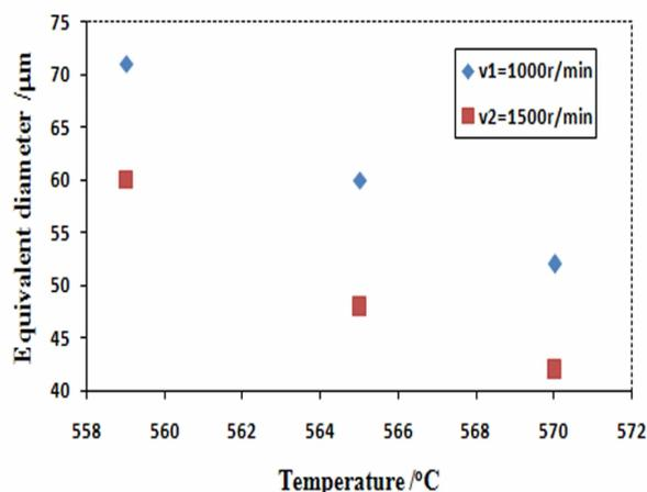
Figure 2 - Equivalent diameters of Si particles versus temperature
