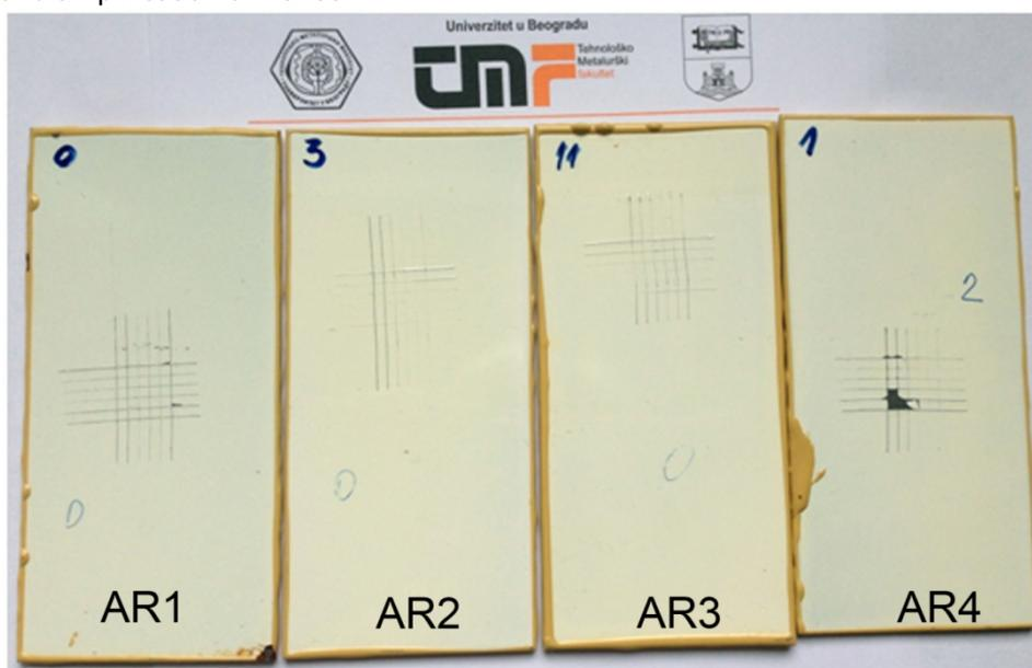
Figure 5 - Dry ARs anticorrosion coating films based on a) AR1 (Co-AR1), b) AR2 (Co-AR2), c) AR3 (Co-AR3) and d) AR4 (Co-AR4) after anticorrosion analysis
