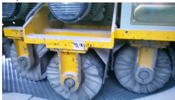
Figure 1 - Polishing rollers rotating around horizontal and central vertical axe in the polishing machine
