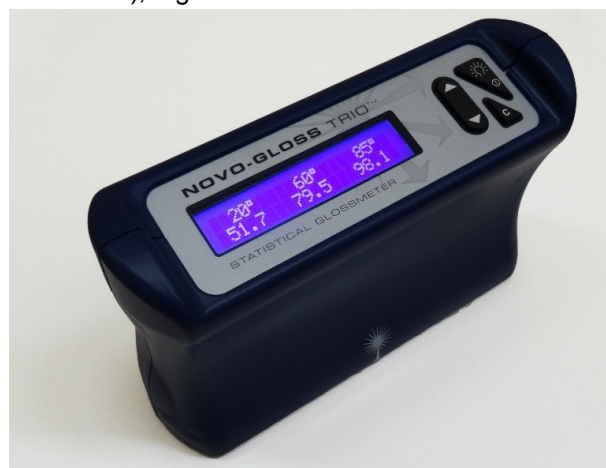
Figure 5 - Determination of the gloss of coated surface
