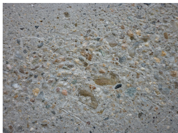
Figure 9 – Surface of the sample of concrete micro-reinforced with polypropylene fiber
