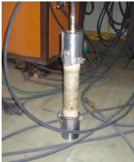
Figure 1 - Metal "cap" fasteners
