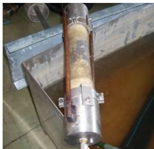
Figure 2 - "Caps" with additional welded bars as reinforcement
