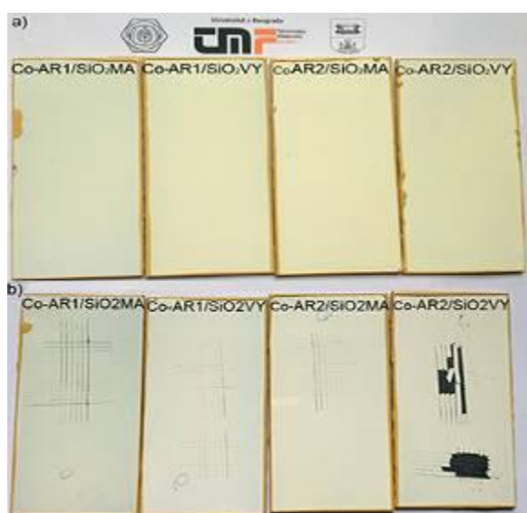
Figure 8 - Dry ARs anticorrosion coating films: Co-AR1/SiO 2 MA, Co-AR1/SiO 2 VY, Co-AR2/SiO 2 MA and Co-AR2/SiO 2 VY a) before and b) after anticorrosion analysis in humid chamber
