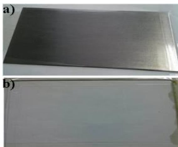
Figure 7 - Alkyd resin based on G-TMP and SiO 2 MA on metal a) and glass plate b)
