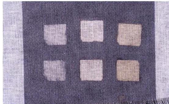
Figure 7. Laser test cleans on artificially soiled new cotton (1.5 cm × 1.5 cm). Upper row (left to right): 1) 266 nm, 0.15 J/cm<sup>2</sup>; 2) 532 nm, 3.2 J/cm<sup>2</sup>; 3) 1064 nm, 2.7 J/cm<sup>2</sup>. Lower row (left to right): 1) 266 nm, 0.1 J/cm<sup>2</sup>; 2) 532 nm, 1.1 J/cm<sup>2</sup>; 3) 1064 nm, 1.0 J/cm<sup>2</sup>
