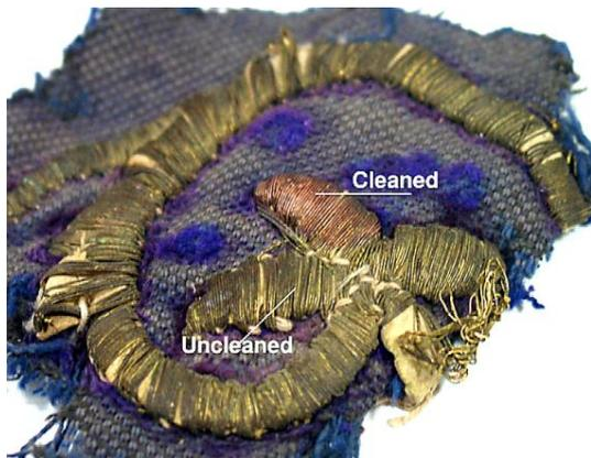
Figure 3. An optical microscopy image shows the surface appearance of the tested metal threads after the laser cleaning
