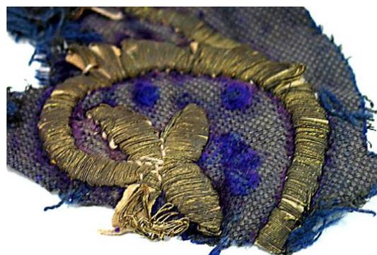
Figure 2. The archaeological Egyptian corroded copper threads at textile
