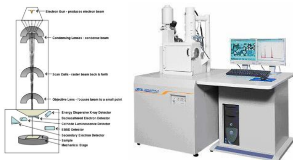
Figure 1. (left) scheme of principles of SEM and (right), image of SEM-EDS instrument used
