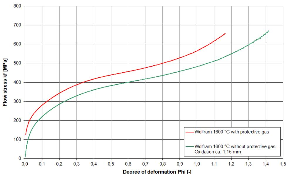
Figure 8. Flow curves of cylindrical wolfram samples at a temperature of 1600 °C: green: heating without protective gas, red: heating with argon atmosphere
