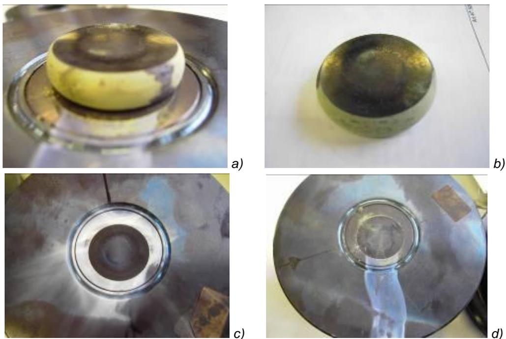
Figure 6. Compressed samples (a, b) and compression tools made of silicon nitride after warm upsetting tests with cylindrical molybdenum and wolfram samples: c) upper tool, d) lower tool
