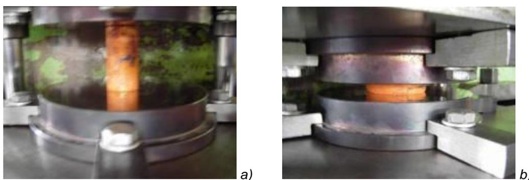
Figure 5. Hydraulic press with compression unit and warm compressed cylindrical sample: a) start of test, b) end of test
