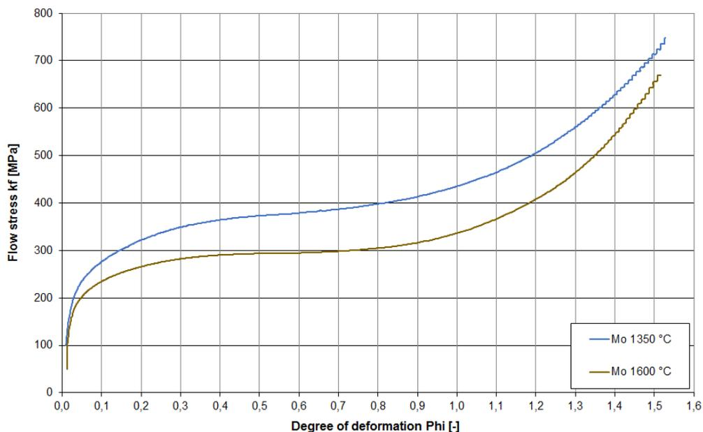
Figure 7. Flow curves of cylindrical molybdenum samples at 1350°C (with protective gas) and 1600 °C (without protective gas)
