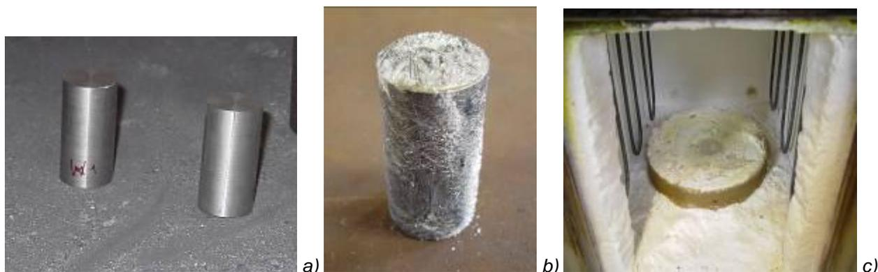
Figure 3. Heating of wolfram and molybdenum samples in a furnace: a – samples before heating; b – molybdenum sample after heating up to 1600°C without protective gas; c – interior of the furnace after heating up of a molybdenum sample without protective atmosphere
