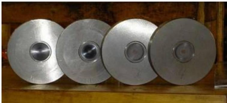
Figure 2.  $\text{Si}_3\text{N}_4$  test samples
