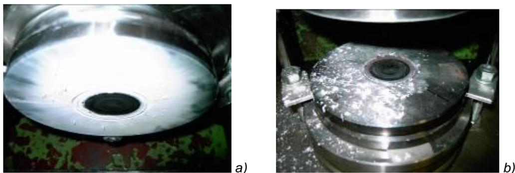
Figure 4. Compression tools made from silicon nitride after warm upsetting tests with cylindrical wolfram samples heated up without protective atmosphere: a) upper tool, b) lower tool
