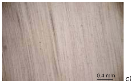
Figure 3. Light microscopy images of the electrode surfaces after cyclic polarization measurements for a) AISI 304, b) AISI 316L and c) duplex stainless steel
