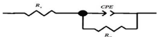
Figure 9. Electrochemical equivalent circuits used to fit the impedance measurements that include a solution resistance ( R_s ), a constant phase element (CPE) and a polarization resistance or charge transfer ( R_{ct} )
