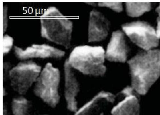
Figure 1. SEM: morphology of Nb powder particles
