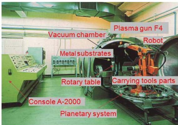
Figure 2. Vacuum plasma spray system
