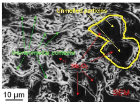
Figure 6. SEM Microstructure of Nb coatings in etched state
