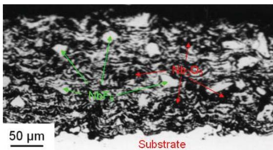
Figure 5. Microstructure of Nb coatings in etched state
