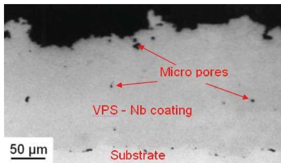
Figure 4. Microstructure of Nb coatings deposited in the state
