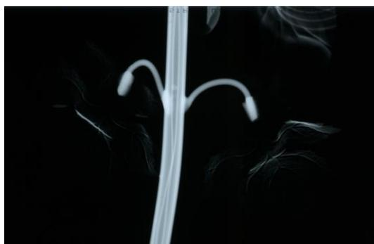
Figure 3. Negative of X-ray film at central part of desk lamp with leaves ( $\approx 1\text{mm}$  in thickness) [9]
