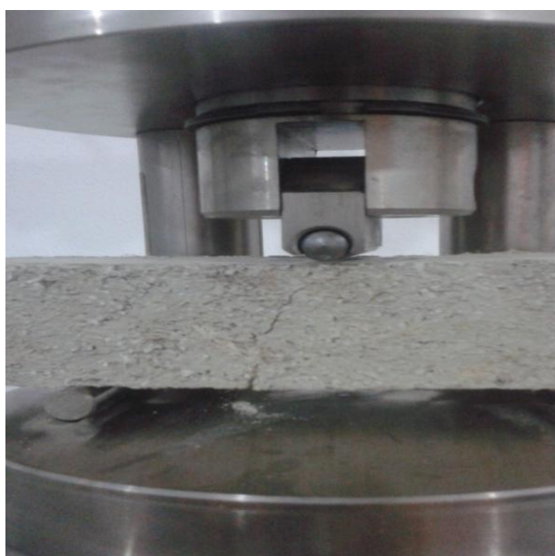
Figure 3. Operation of testing the flexural strength of composite sample
