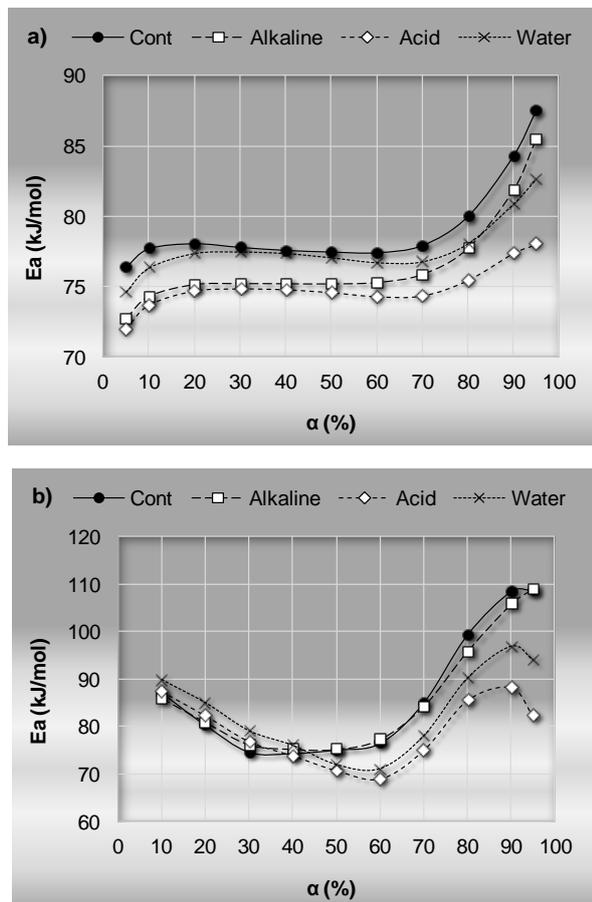
Figure 1. Activation energy ( $E_a$ ) dependance on conversion obtained by KAS (a) and Friedman (b) methods for the curing of different UF adhesive systems with wood flour: control (non-treated wood flour); alkaline (wood flour treated with sodium carbonate); acid (wood flour treated with acetic acid) and water (wood flour treated with distilled water)
