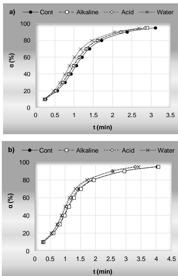
Figure 2. Conversion degree in function of time at the constant temperature of 80°C obtained by KAS (a) and Friedman (b) methods, for the UF adhesive systems with wood flour: control (non-treated wood flour); alkaline (wood flour treated with sodium carbonate); acid (wood flour treated with acetic acid) and water (wood flour treated with distilled water)
