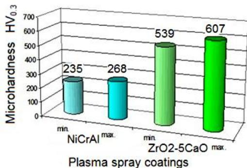
Figure 2. Microhardness of  $ZrO_2$ 5CaO/NiCrAl coating
