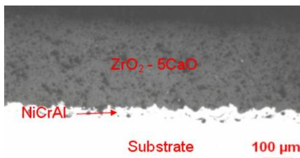
Figure 3. The microstructure of  $ZrO_2$ 5CaO/NiCrAl coatings
