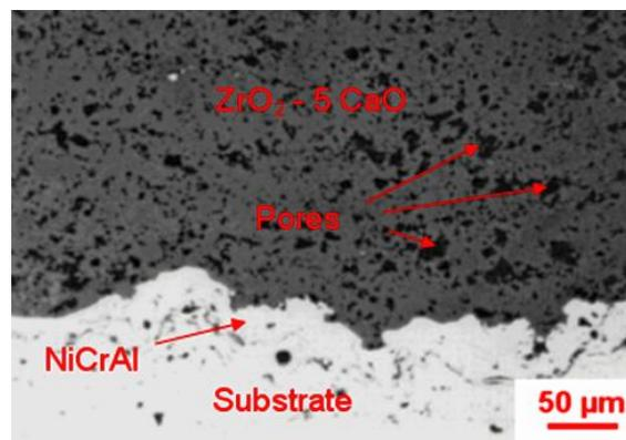
Figure 4. The microstructure of  $ZrO_2$ 5CaO/NiCrAl coatings
