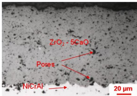
Figure 5. The microstructure of  $ZrO_2$ 5CaO/NiCrAl coatings
