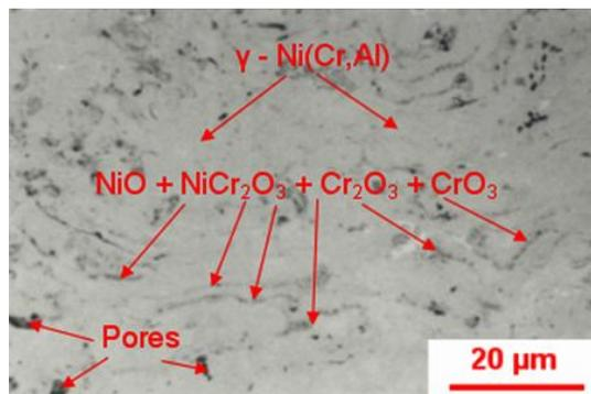
Figure 6. The microstructure of  $ZrO_2$ 5CaO/NiCrAl coatings
