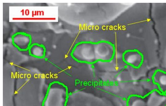
Figure 7. (SEM) Surface morphology of the  $ZrO_2$ 5CaO coating
