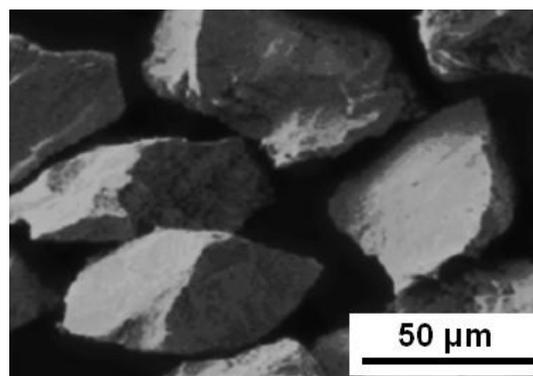
Figure 1. (SEM) micrograph of the  $ZrO_2$ 5CaO powder particles
