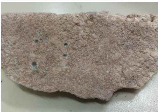
Figure 3. Mortar sample ( \approx 5 cm long) subjected to analysis with microdamages provoked by LIBS
