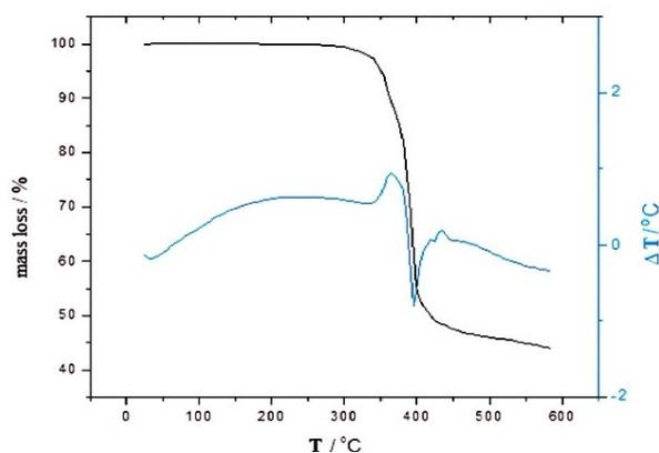
Figure 3. Simultaneous TG-DTA of  $[\text{Co}_2(\text{Cl})_2\text{tpmc}](\text{BF}_4)_2$ .
