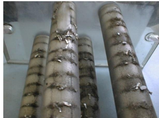
Figure 1. Material contamination on the magnetic separator of the granulate bunker
