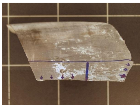
Figure 13. Material from the screw flights. The marking shows the point at which the specimens were taken (a) and the fracture surface in the transverse direction (b)
