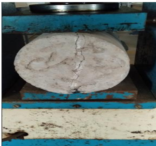
Figure 11. Split tensile strength test
