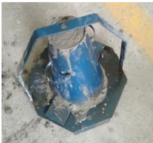
Figure 7. Slump cone test
