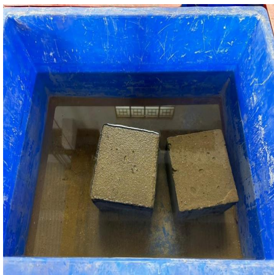
Figure 17. Sulphate attack test
