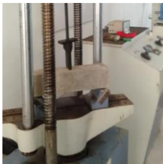
Figure 13. Flexural strength test
