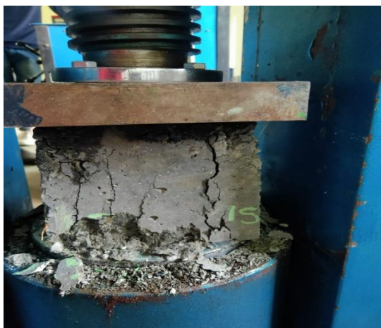
Figure 9. Compressive Strength Test
