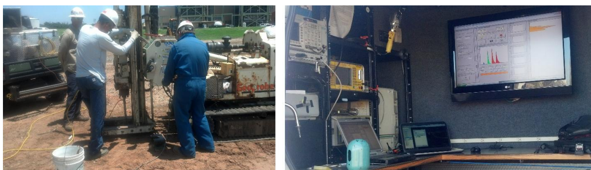
Figure 2. The screening performed by pushing probe into the soil, while the LIF system displayed in real-time LNAPL fluorescence occurrence
