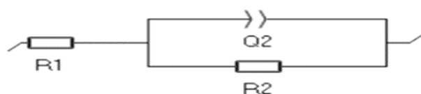
Figure 3. Electrical equivalent circuit used to fit the EIS parameters of the carbon steel in 3.5wt% NaCl without and with the MPL inhibitor
