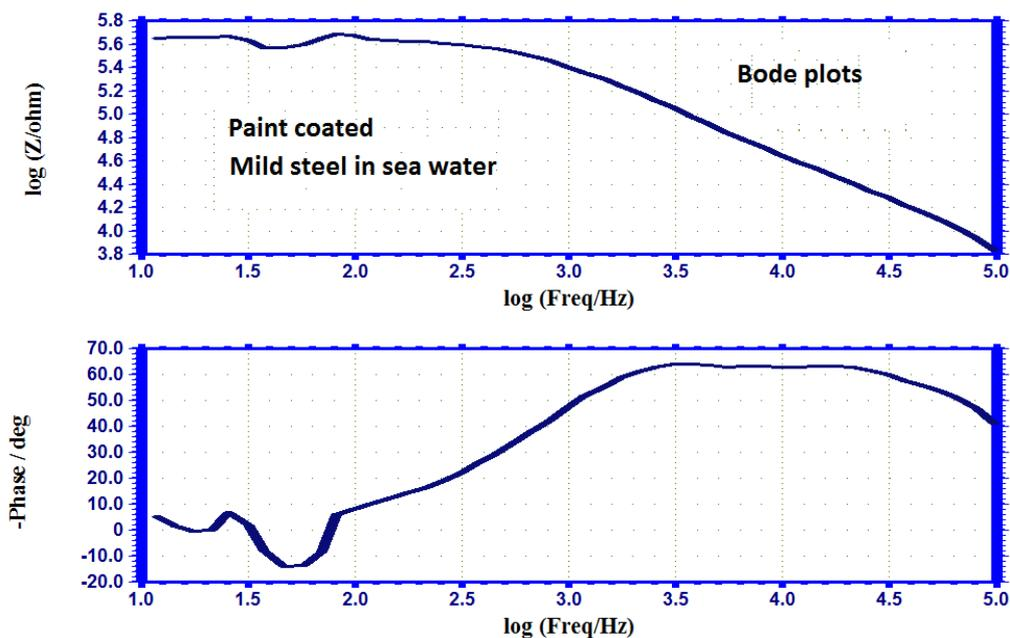
Figure 10. Bode plot of paint coated mild steel in seawater
