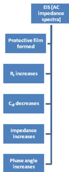
Figure 5. Correlation among corrosion parameters of AC impedance spectra
