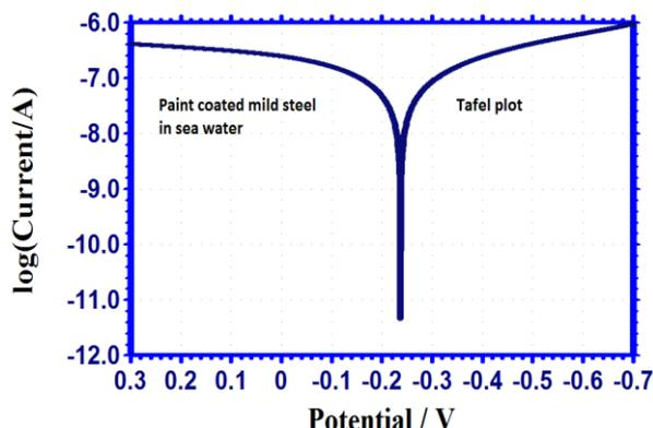
Figure 3. Polarisation curve of paint coated mild steel in seawater
