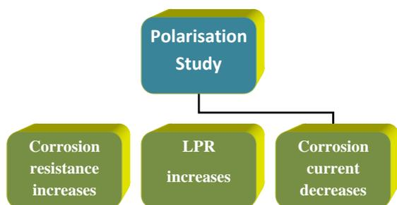
Figure 4. Correlation among corrosion parameters of polarization study
