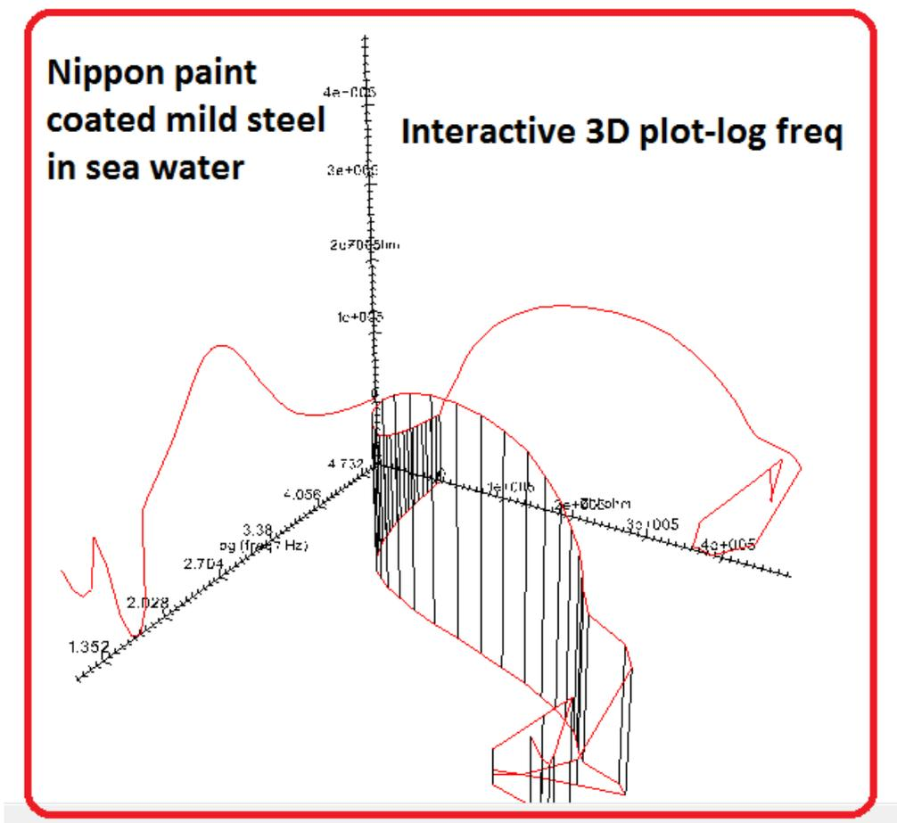
Figure 11. Interactive 3D-log freq plot of paint coated mild steel in seawater
