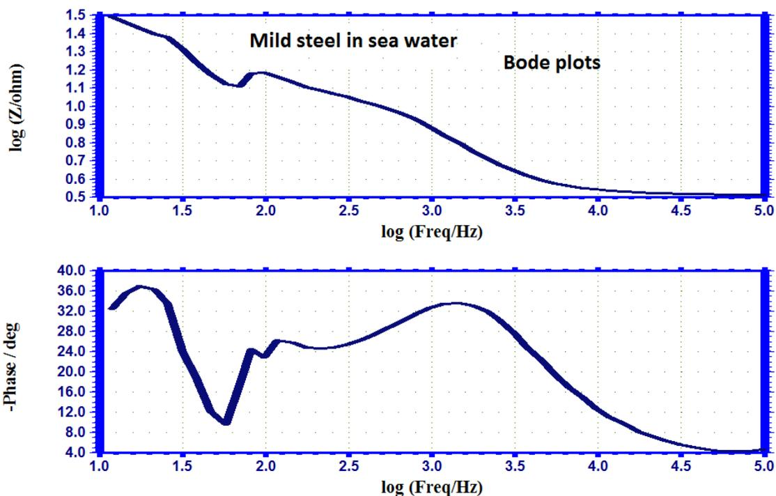
Figure 7. Bode plot of mild steel in seawater
