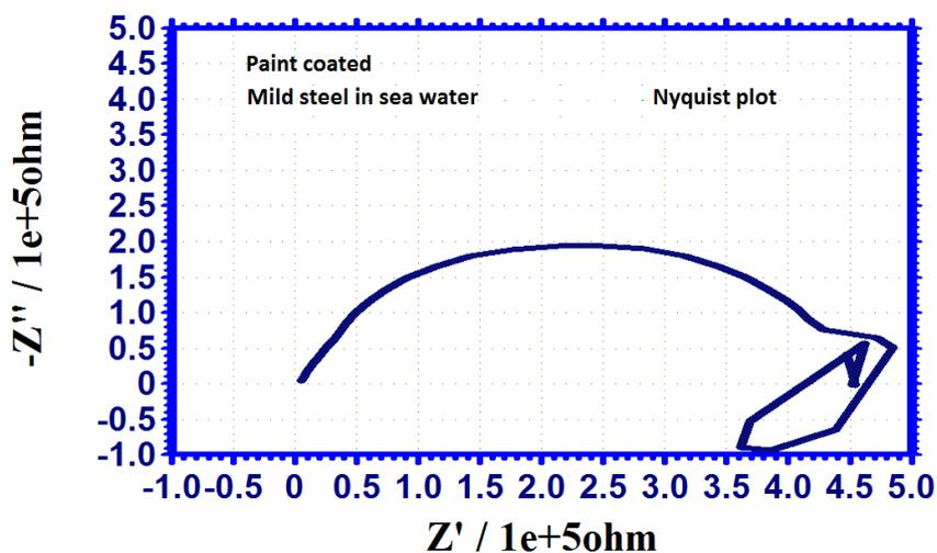
Figure 9. Nyquist plot of paint coated mild steel in seawater
