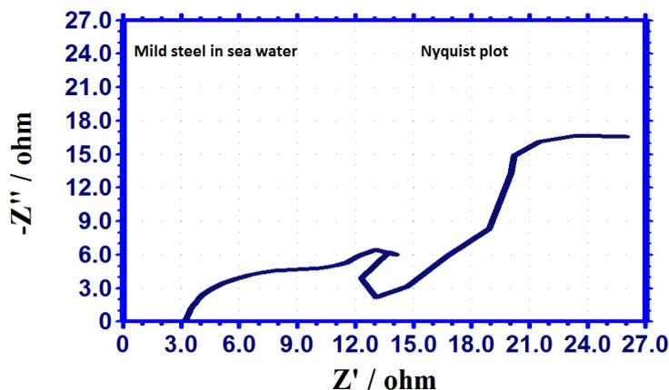
Figure 6. Nyquist plot of mild steel in seawater
