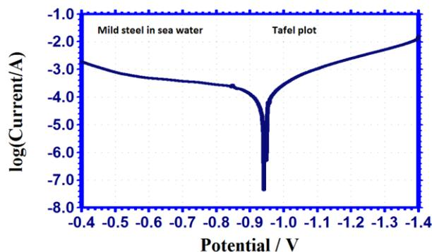
Figure 2. Polarisation curve of mild steel in seawater
