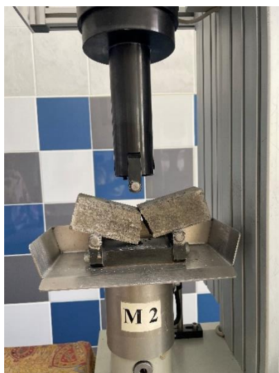
Figure 8. Determining of flexural strength
