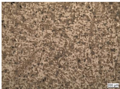
Figure 5. Microstructure graphitized HSS [50]
