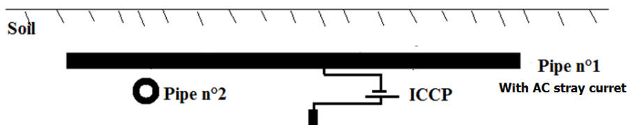
Figure 5. Schematic representation of the system employed to assess the influence of combined AC and DC stray currents on cathodic protection performance
