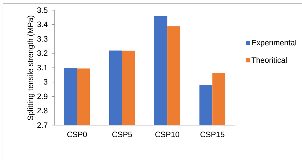
Figure 7. Comparison of Experimental and theoretical split tensile strength of POFA supplemented CS concrete
