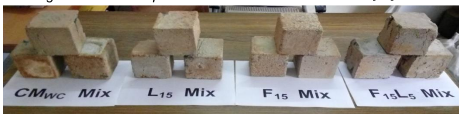
Figure 13. Specimens after 180 days submergence in HCl solution
