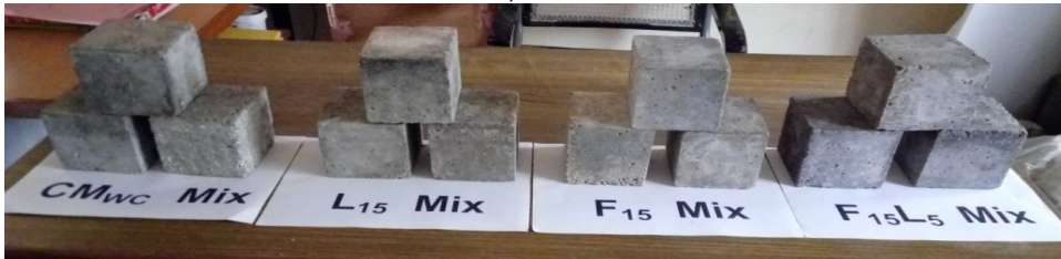
Figure 16. Specimens after 180 days immersion in NaCl solution
