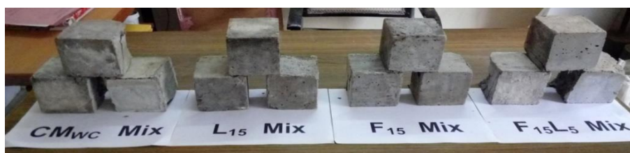
Figure 10. Specimens after 180 days submergence in MgSO_4 solution
