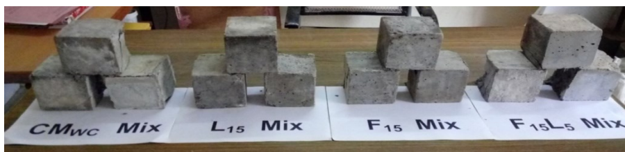
Figure 10. Specimens after 180 days submersion in MgSO_4 solution
