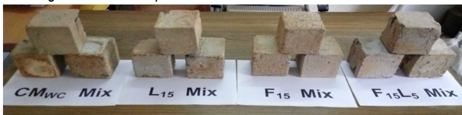
Figure 13. Specimens after 180 days submergence in HCl solution
