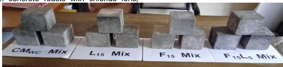
Figure 16. Specimens after 180 days immersion in NaCl solution
