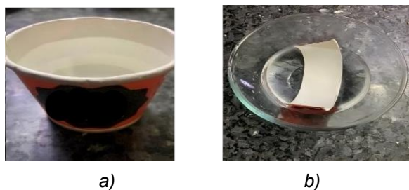
Figure 2. (a) Hot water was poured and left undisturbed for 15 minutes in each cup for MP leaching. (b) The cup was cut and dipped in hot water for the separation of plastic film from the inside of the cup
