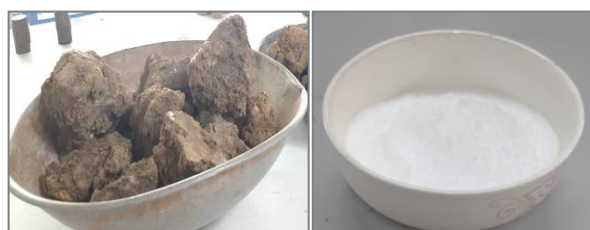
Figure 1. (a) Soil (b) Nanosilica
