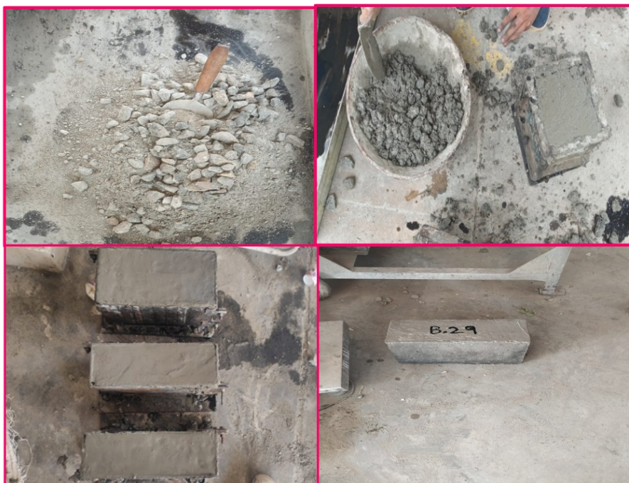
Figure 5. Casting of Conventional Block and LWC block
