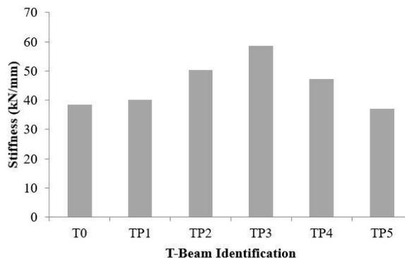
Figure 6. Stiffness of Control and PVCC Nano layered T-Beams
