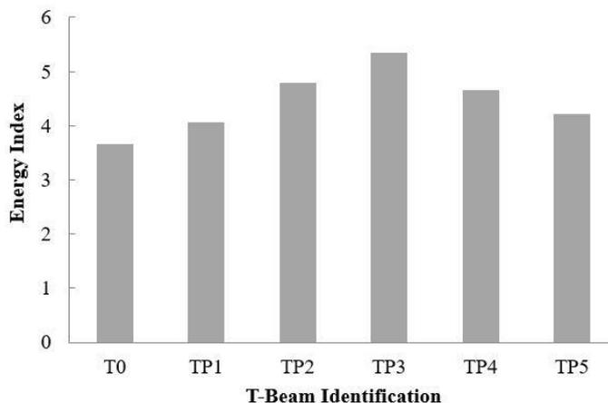
Figure 8. Energy Index of Control and PVCC Nano layered T-Beams
