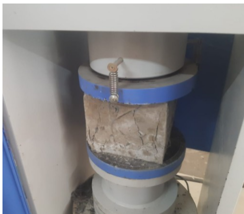
Figure 4. Test Set up for Compressive Strength
