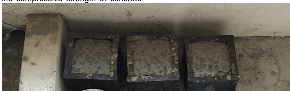
Figure 3. Casting of Cube
