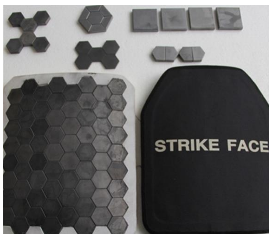
Figure 2: Hard armour panel made up of silicon carbide
