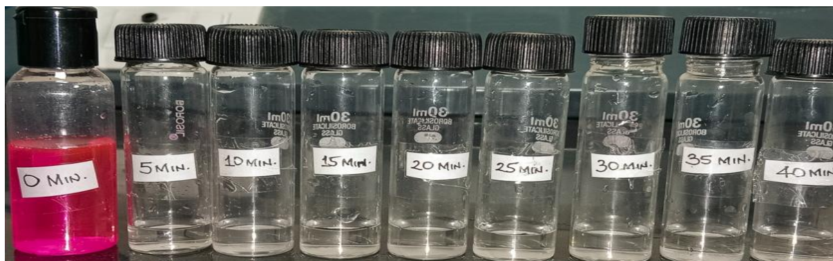
Figure 9. RhB Dye Adsorption utilizing ZnO-rGO NC for 5–40 min.
