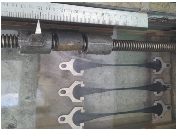
Figure 3. Determination of the bitumen extensibility (ductility)
