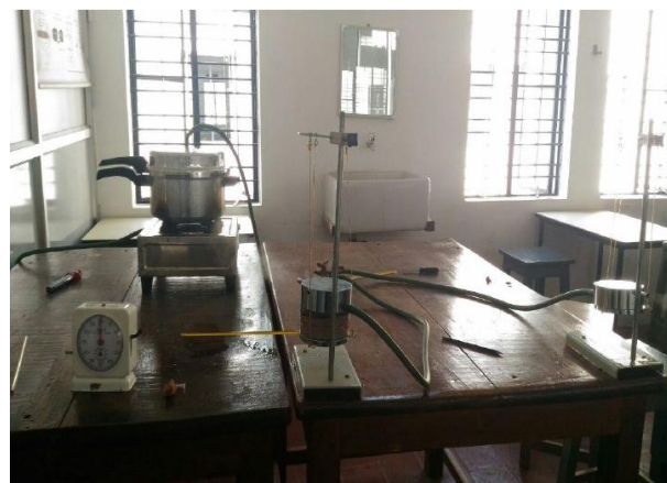
Figure 6. Lee's Disc Apparatus Setup
