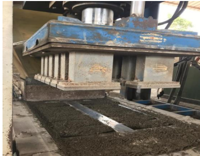
3e) Compacting the brick
