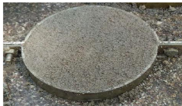
Figure 3. Manufacturing of Straw Sandwiched Fly ash Brick
