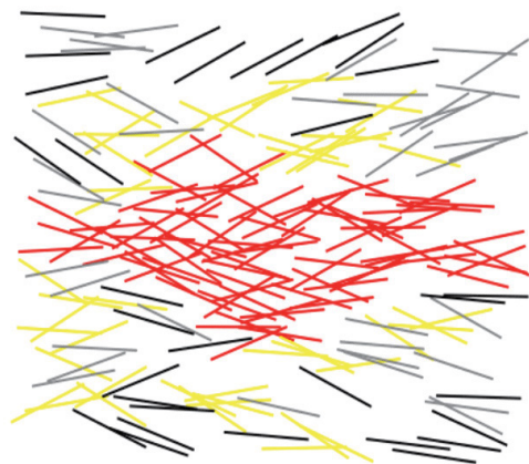
Figure 3. Distribution of carbon nanofibers in the polymer matrix (the filler concentration is 8%): red – the percolation cluster, yellow - long chains of interacting particles in the absence of a percolation cluster, gray - interacting particles not included in long chains, black - non-interacting particles.
