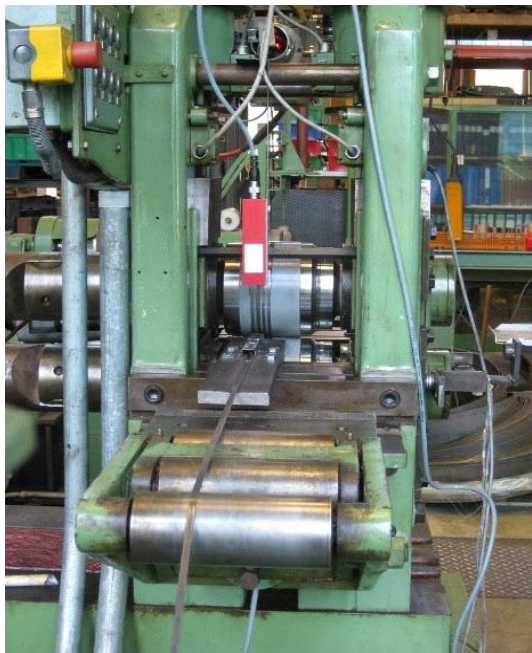
Figure 9. Cold rolling test with \text{Si}_3\text{N}_4 compound rolls
