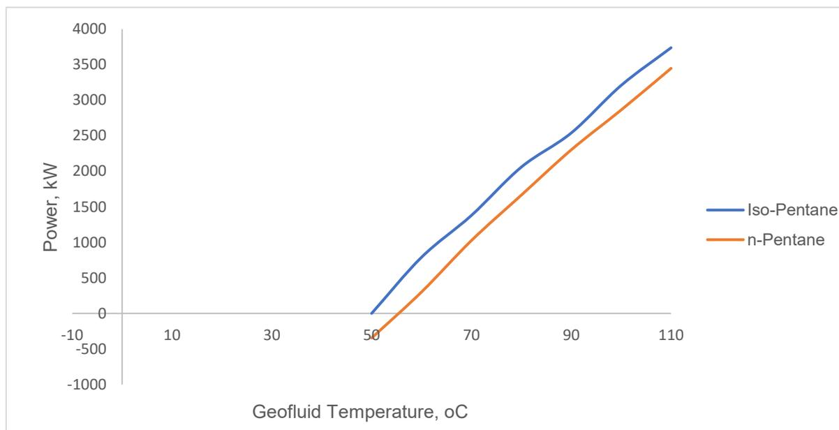
Figure 7. Effect of geofluid temperature on power produced using CO<sub>2</sub> as geofluid at 80 kg/s
