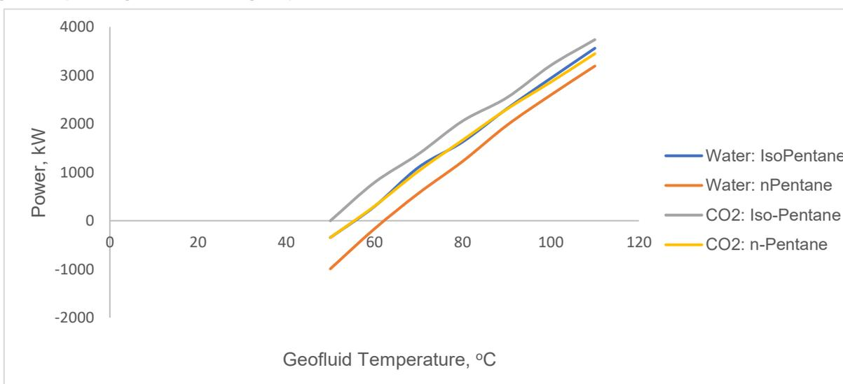
Figure 10. Effect of Geofluid on power production using water and CO<sub>2</sub> geofluids
