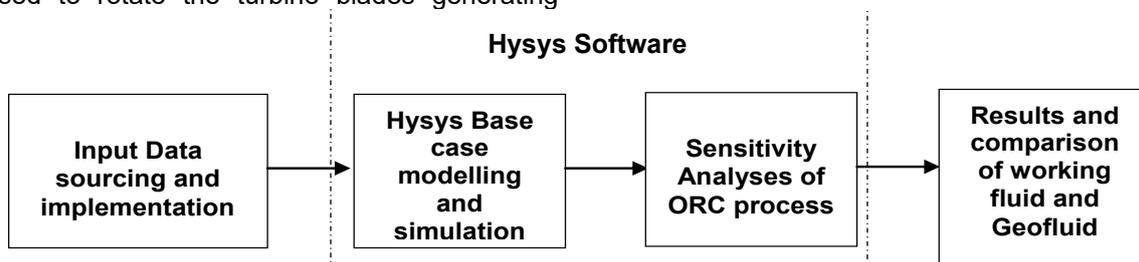
Figure 2. Simulation Process Block Diagram
