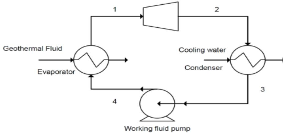
Figure 1. The working principle of the ORC system
