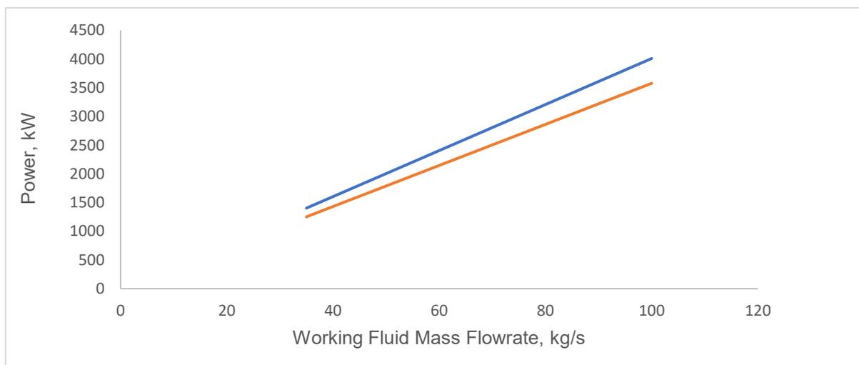
Figure 9. Effect of mass flowrate on power production using CO<sub>2</sub> as geofluid at 100 °C
